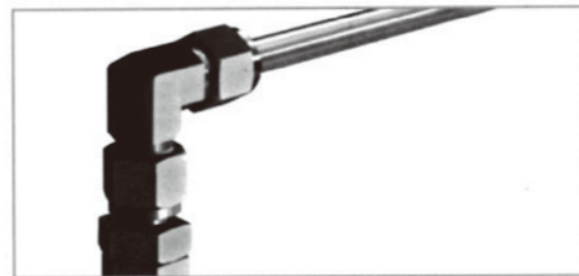
4. Connect union elbow to adapter by tightening EMT connection with wrench while holding elbow pointing in desired direction Then insert tubing into the other end of the Union Elbow and connect tubing
