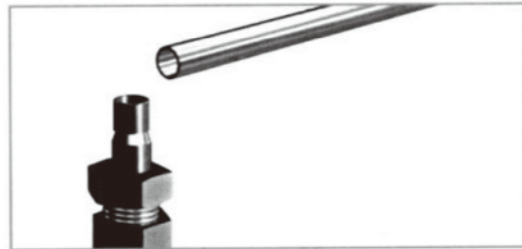
3. To connect this situation, merely tighten pipe thread of male adapter into female port.
